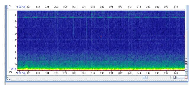
**Figure 4.** An example of light electrical noise coming through the hydrophone recordings. Recordings like this were acceptable for use in the statistical sampling.
