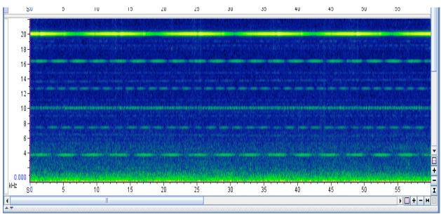
**Figure 3.** An example of electrical noise coming through the hydrophone recordings. Recordings like this were not used in the statistical sampling.
