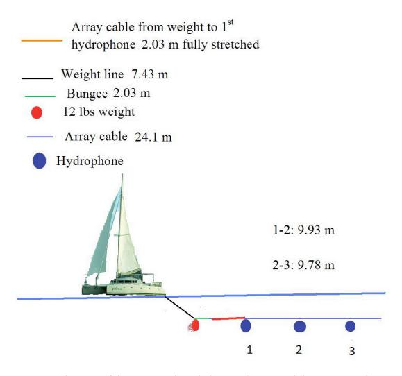
Figure 1: diagram of the Gato Verde with the towed array and the positions of its various elements.
