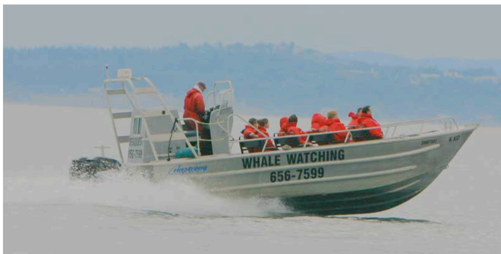
Figure 5. K-KO is a twelve-passenger whale watching boat with twin 225 Hp outboards.
