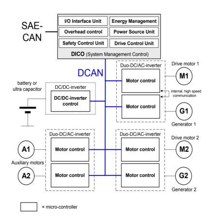
Modular concept, whereby configuration of the application is programmed in the DICO
