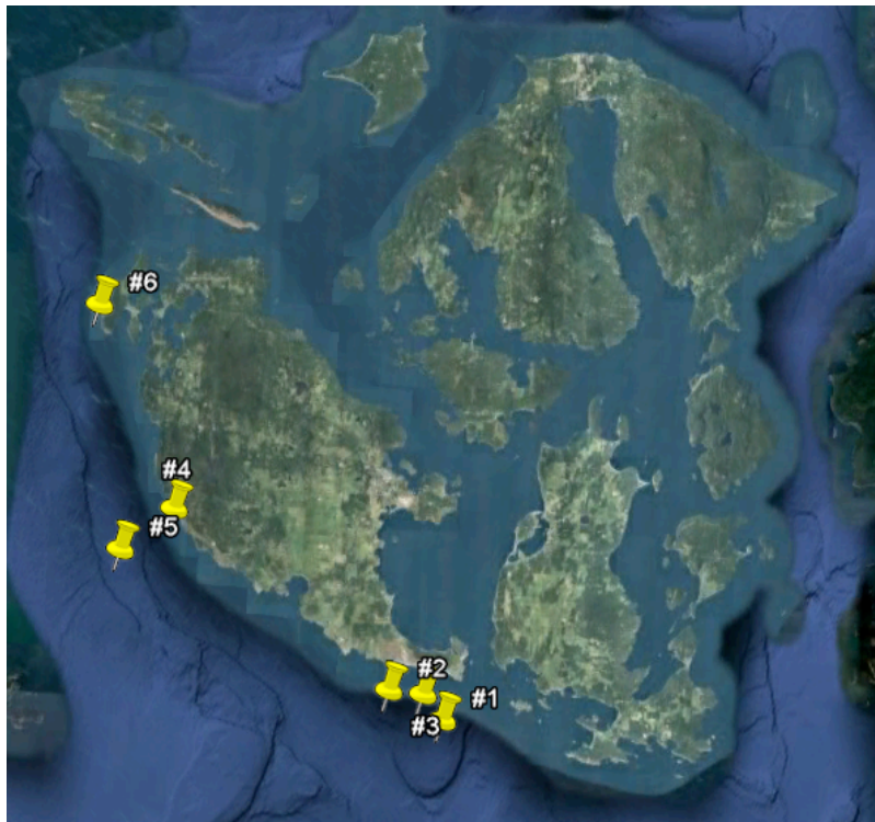
Figure 1. Proposed study sites to measure sound propagation. Sites #1, #2, and #3 are shallow water sites with sand/gravel bottoms. #1 and #3 are low relief sites, while #2 lies on a slope. Site #4 is along a steep, rocky slope. Sites #5 and #6 are deepwater sites with rocky bottoms.
